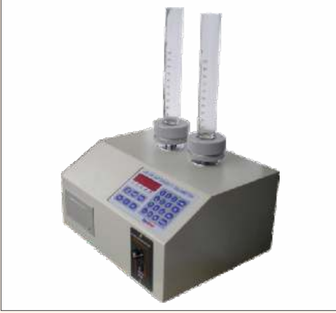
Figure 8: (A) Bulk Density measurement unit (B) Tapped density measurement unit
