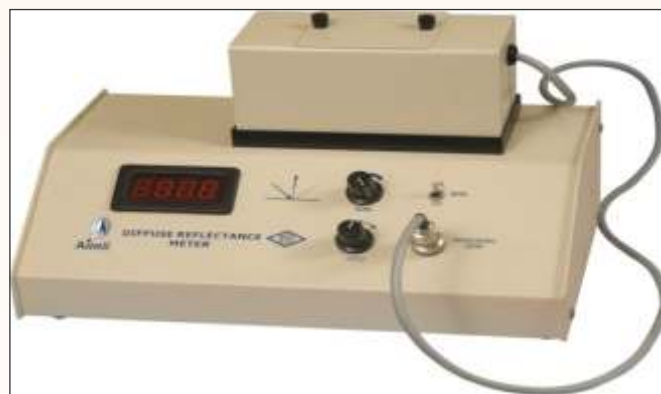
Figure1: Diffuse Reflectance Meter for measurement of whiteness, brightness and opacity of minerals
