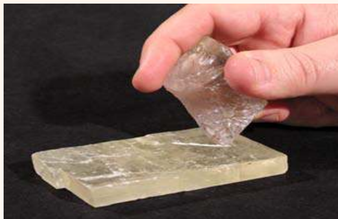
Figure 4: Testing mineral hardness. The harder mineral (quartz) scratches the softer one (calcite)
