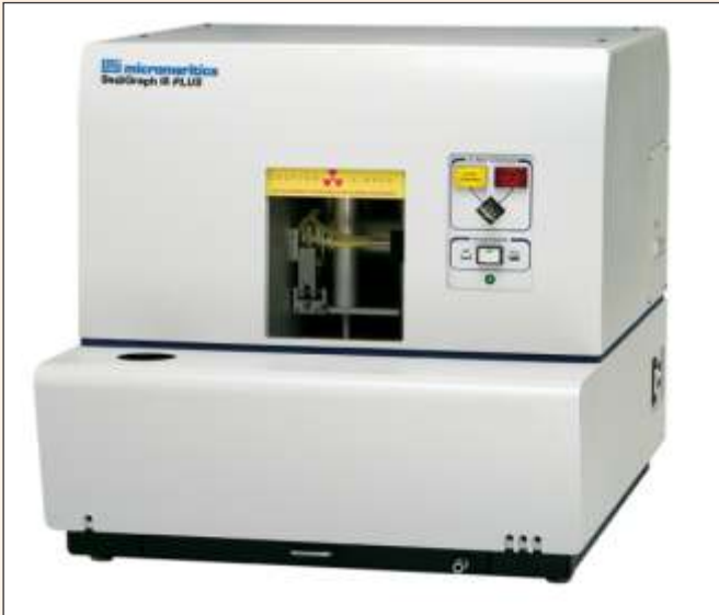
Figure 5: Sedigraph instrument for measurement of mineral particle size
